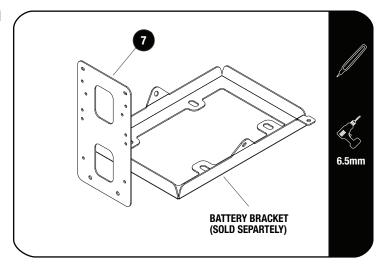
Determine where on the Battery Bracket you would like to mount the Battery Device Mounting Plate (Item 7). Using a marker pen, mark the two holes.
