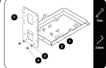
Using two M6 x16 Countersink Screws, two M6 x 19 x 1SS Flat Washers, two M6 x 12 x 1SS Flat Washers and two M6 Nyloc Nuts (Items 1, 2, 3 & 4) fasten the Battery Device Mounting Plate (Item 7) to the Battery Bracket.
